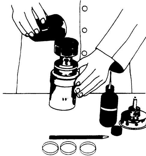
Figure 3-D Pouring the measured water sample into the funnel
